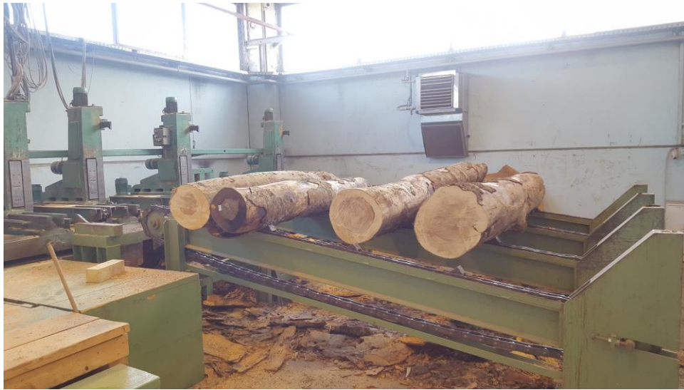
Slika 2. Transport trupaca trakastim transporterima
